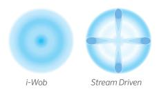
In this example, the i-Wob is instantaneously spreading the same amount of water over an area five times greater than the area covered by the spray nozzle.
