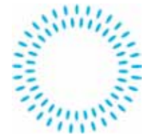
Double Pad: 66 Streams 3.93 - 11.5 gpm (893 - 2619 L/hr)
