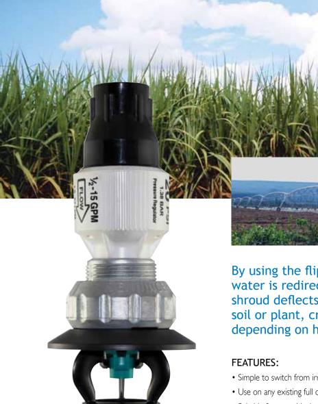
By using the flip side of the LDN® pad, the water is redirected up into the shroud. The shroud deflects the water down toward the soil or plant, creating a 36" diameter of water, depending on height above the ground.
